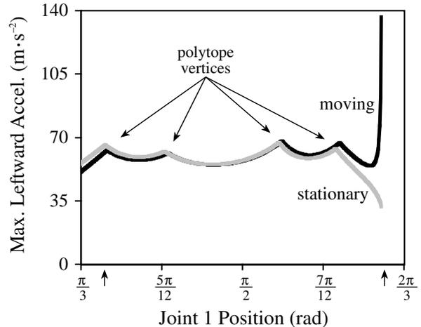
Fig. 4. Maximum leftward acceleration achievable at each position of joint 1. Shown are two conditions where the manipulator is stationary (gray curve) or moving (black curve). Local extrema occur whenever the active torque constraint changes at a polytope vertex. Small arrows mark the values of  $q_1$  that correspond to the configurations shown Figure 3.
