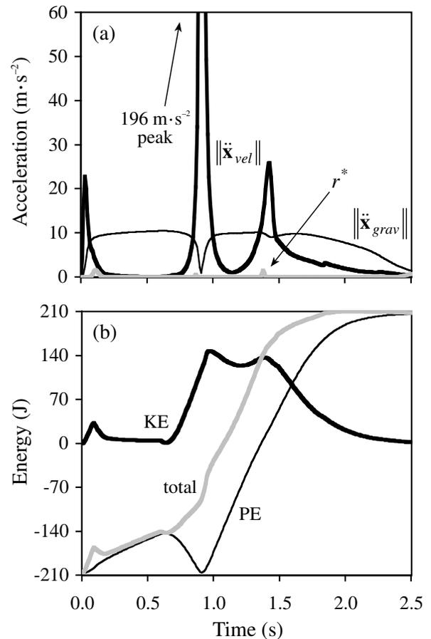
Fig. 6. Acceleration (a) and energy (b) versus time for the trajectory illustrated in Figure 5. Shown in the upper plot (a) are the acceleration radius (gray curve, barely visible) and the magnitude of the acceleration offsets due to gravity and velocity (light and heavy curves, respectively). Shown in the lower plot (b) are potential, kinetic, and total energy during the movement (light, heavy, and gray curves, respectively).
