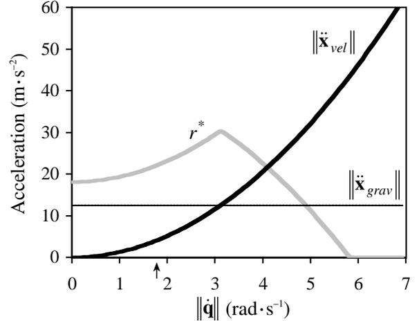
Fig. 2. Acceleration versus joint velocity magnitude with  $\dot{q}_1 = \dot{q}_2 = \dot{q}_3 = \omega$ . Shown are the acceleration radius (gray curve) and the magnitude of the acceleration offsets due to gravity and velocity (light and heavy curves, respectively). The small arrow marks the value of  $\|\dot{\mathbf{q}}\|$  that corresponds to  $\omega = 1$  as in Figure 1.
