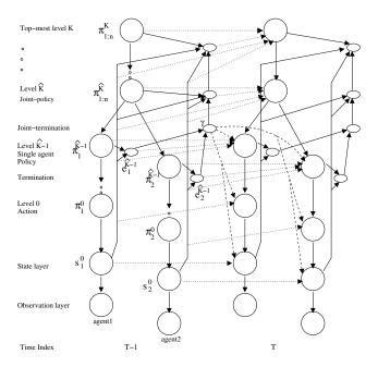
Figure 5: The DBN representation showing two agents. Each agent policy hierarchy is an AHMM with  $\hat{K}$  levels.  $\gamma$  at level  $\hat{K}-1$  is the coordination node. In the  $T_{all}$  scheme, the dashed arcs from  $\gamma_t$  to the single agent policies below level  $\hat{K}-1$  are removed. The dotted-arcs represents the inter-time slice dependency.
