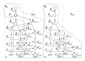
Figure 8: Belief state updating from  $\mathcal{B}_{t+}$  to  $T_{t+1}$ . All marginals of  $\mathcal{B}_{t+}$  above the highest level of termination are retained in  $T_{t+1}$  a. shows update procedure when the highest level termination is  $\geq \hat{K}$ . b. shows update procedure when no joint policies have terminated. Here agent 1 has its highest level of termination at level  $\hat{K}-2$  and agent 2 at level 0
