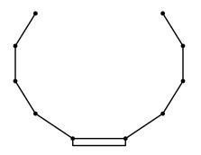
Figure 3.4. Schematic of "robot" used in simulations. Robot is planar and has a total of 10 DOFs. The base is mobile and can move vertically and horizontally. Each arm has four rotational joints, and no joint limits are imposed. Each arm link is one unit in length, and the base is a rectangular box which is one unit wide and 0.2 units high. This design is inspired by designs used in Jordan (1992); Jordan and Rumelhart (1992); Jordan (1990, 1988).
