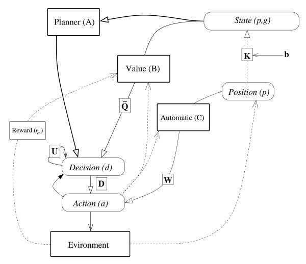
**Figure 4.3.** Architecture of the connectionist-style model. Unfilled closed arrows indicate excitatory connections, filled closed arrows indicate inhibitory connections, and open arrows indicate unrestricted connections. For clarity, ascending projections are shown with dashed lines. Arrays of neurons are represented by boxes with rounded corners and labeled with italics.
