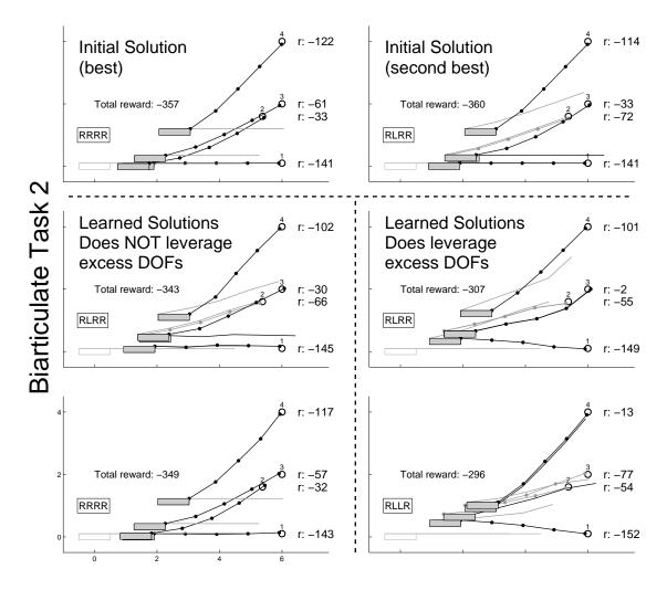
Figure 3.11. Follows the same conventions as in Figure 3.9. However, the reward for each movement is indicated to the right of the goals, as in Figure 3.5. Dashed lines separate three sets of solutions. The top set indicates initial solutions for two different sequences of hand recruitment. The bottom left set indicates learned solutions in which excess DOFs are not leveraged (see text). The bottom right set indicates learned solutions in which excess DOFs are leveraged.
